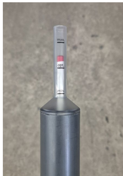
Water Level Gauge
